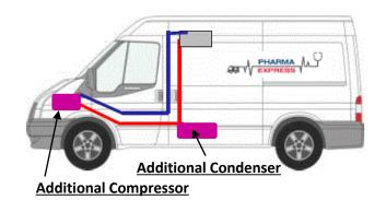
The Pharma Power Plus system **is complete independent** from the vehicle original HVAC system with a additional Pharma compressor and undermount condenser.
